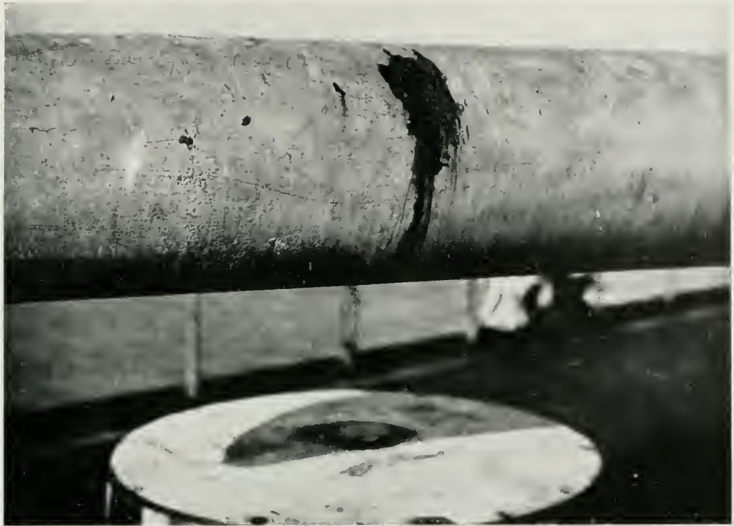
EXPANSION RING MARKING ON 6-INCH GUN "NURNBERG."
